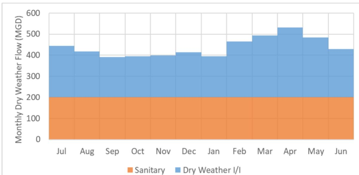
Figure 8: Collection System Monthly Dry Weather Flow FY2018. Source: GLWA WWMP.
